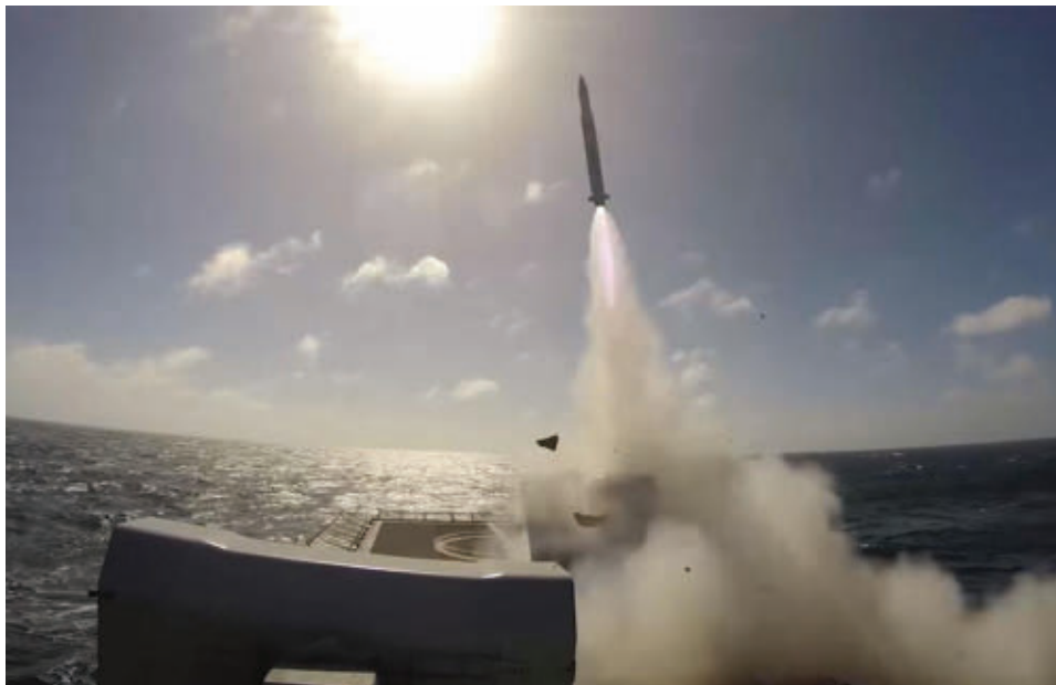
RIM-162 Evolved Seasparrow Missile (ESSM) Block 2 has a dual-mode X-band radar seeker than can engage enemy planes and missiles at ranges beyond 25 miles.
