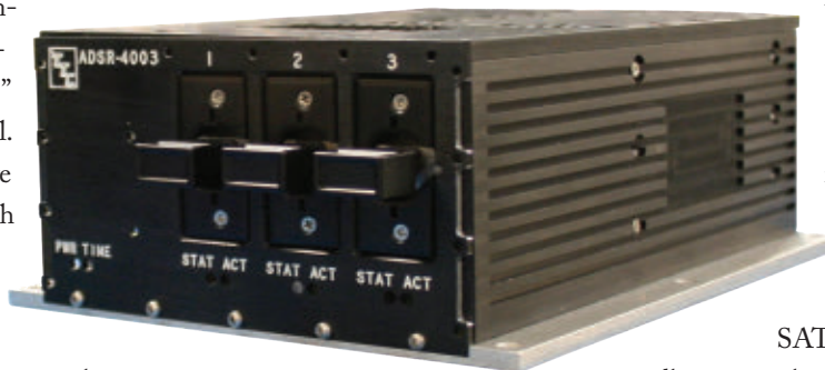
▲ The ADSR-4003-1 data recorder from The Curtiss-Wright TTC business unit is an instrumentation recorder with a built-in file server capability, two 1000 BASE-T Ethernet ports, and as many as three removable solid-state memory cartridges.
